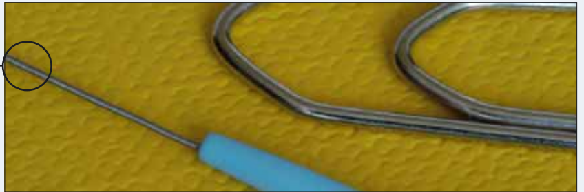
Close-up of a catheter and guide wire. The wire is 0.3 mm thick, and the catheter has a diameter of 1.6 mm. In a recess at its tip, the guide wire carries a piezoresistive sensor to measure blood pressure (see the two images below). (Radi Medical Systems, Pressure Wire)
