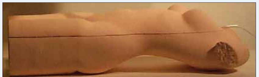
For her tests Tanase used a life-size patient dummy with a model of the aorta and the main arteries in the legs (see opening picture). The dummy was constructed at the Electrical Engineering faculty workshop.
