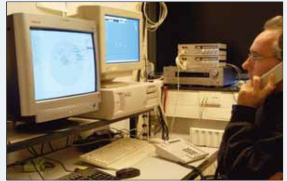
The room for observing the intelligent living room contains the telephone server (on the right) and the atmosphere controller (left).
