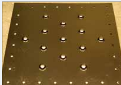
In his experimental set-up, researcher Leon Geers used plates with jet nozzles in a matrix similar to that used in the ovens made by Rademaker Den Boer.
